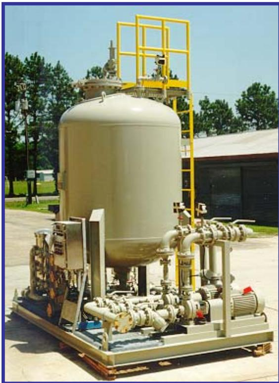
**Potable water pressurization set** for a chemical plant in Nigeria. This pump and tank set was built to oil field specifications. A unique feature of this skid is the large (1500 gallon) bladder tank. The bladder was custom fabricated.
