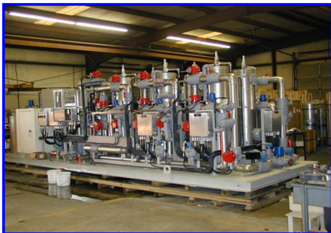
Skid Mounted-Stainless Steel Pipe-Insulated and Heat traced. PLC Controlled
